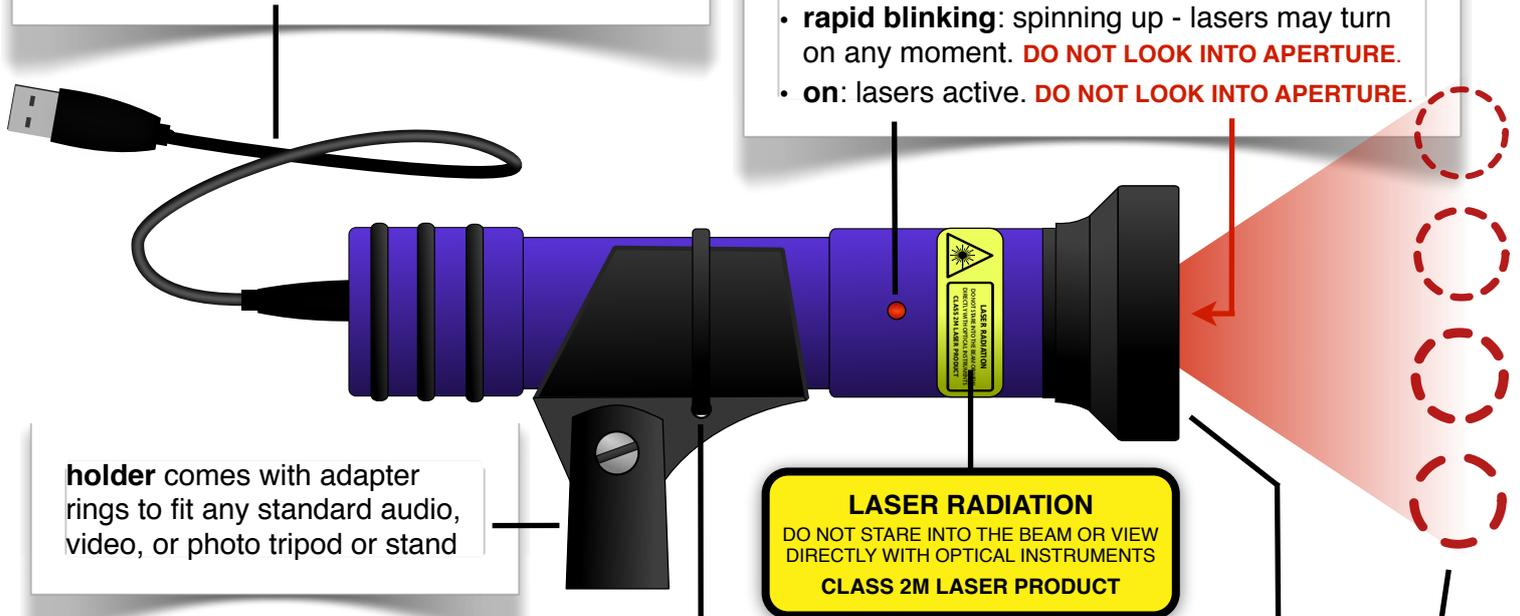
**holder** comes with adapter rings to fit any standard audio, video, or photo tripod or stand
